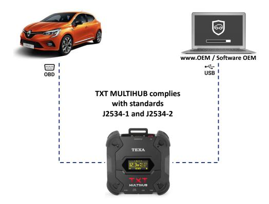
The Pass Thru SAE J2534 standard aims to ensure that specific ECU diagnosis and reprogramming operations can be carried out via a third-party VCI.
